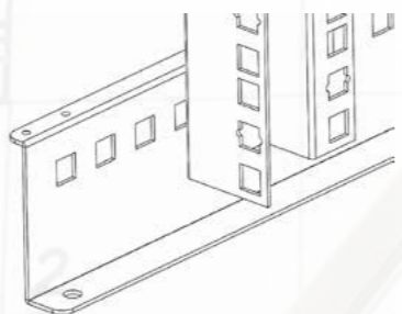
19" Mounting rail and Z-shape Horizontal bar
