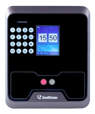
The face recognition reader can work with GV-AS Controller and GV-ASManager for an intuitive, smart access control solution. When integrated with GeoVision controller and software, GV-FR2020 can operate under Face Recognition mode, as well as other modes including Card, Card + Face Recognition and Password + Face Recognition.
