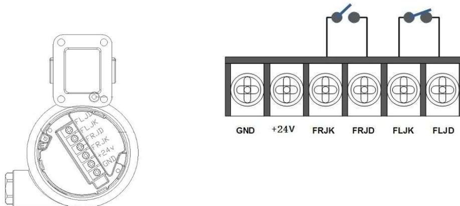
**FLJD/FLJK** : Normally closed contact output of the fault relay;
